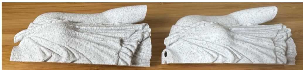
Figure 28: Upper Body piece printed in the fuzzy skin texture (left) and normal texture (right)
