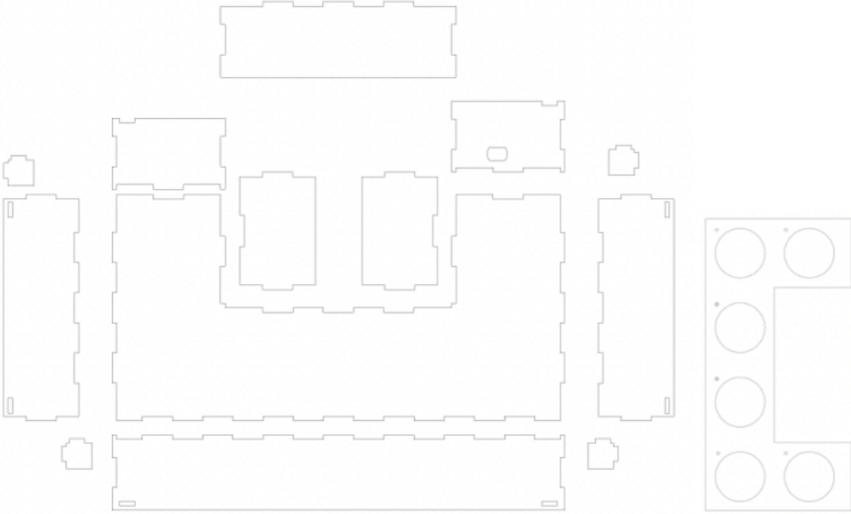
Figure 40: 2D vector drawing of the Base
