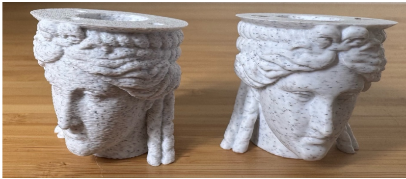
Figure 29: Head piece printed in the fuzzy skin texture (left) and normal texture (right)
